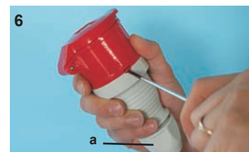
To disassemble first unscrew the cable gland (a). Then press the screwdriver (blade width 3.0 mm) deeply into the opening slot of the back part. Turn screwdriver clockwise to unlock the parts again.
