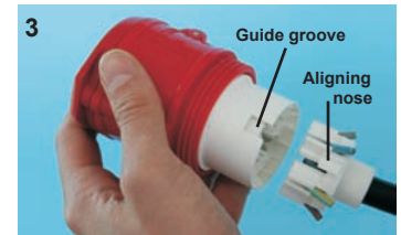
Fit distributor ring onto front part. Important: Aligning nose provides for correct position when inserted in guide groove.
