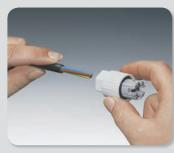
Lead the cores into the marked core entries and cut off the projecting core ends flush, i.e. so that there is no overhang.
