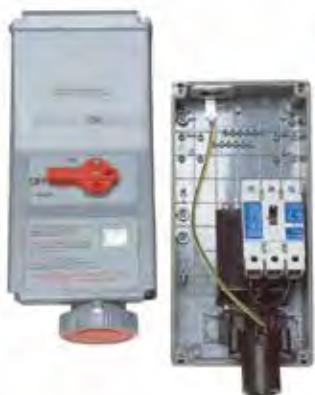
The Circuit Breaker Mechanical Interlock integrates a circuit breaker (which takes the place of a switch) and receptacle in a non-metallic enclosure that meets NEMA type 4X (Washdown, Corrosion Resistant) requirements.
