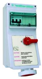
Walther Mechanical Interlocks, with built-in circuit breakers, incorporate an interlocking receptacle with MCB Type "C" circuit breakers in a nonmetallic enclosure that meets Type 4X (Washdown, Corrosion Resistant) requirements.
